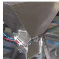
Discharge chute + timing hopper
